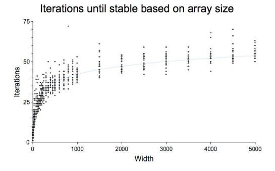
After becoming stable, the percentage of elements completely surrounded by those of like spin was calculated. For grid sizes of about 100x100 or larger, the final 'domain size' of the material becomes remarkably constrained:
