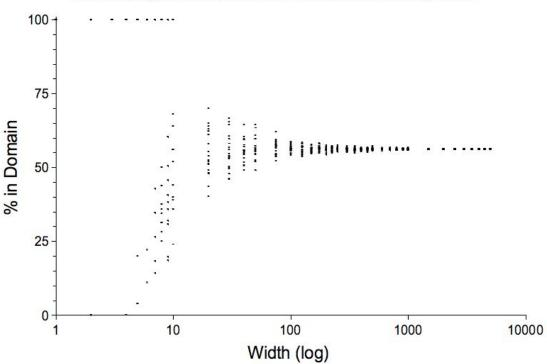
Percent of elements in a domain when stable, based on size of model
